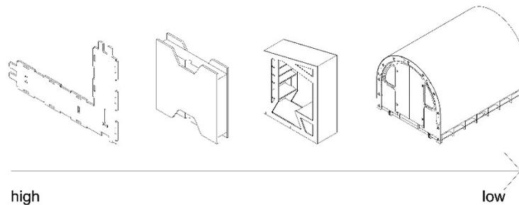
Figure 5: Module size and customizability of different approaches From left, each component part of projects such as the WikiHouse and Facit Homes is parametrically flexible. With Blokaloks, the module is a given, but its aggregation is variable; whereas the PlyPAD has a much larger “programmatic module.” Finally, Shelter 2.0 and the D1 house offer single, standard designs.
