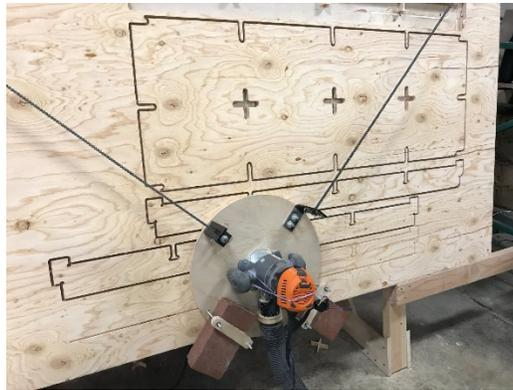
*Figure 7: The Maslow CNC cutting parts for the PlyPAD*
